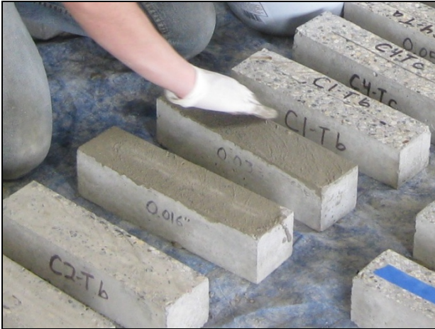
Figure 6. Hand application of the hydraulic cementitious material
