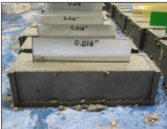
Figure 5. Durability Test Specimens with Metal Shims
