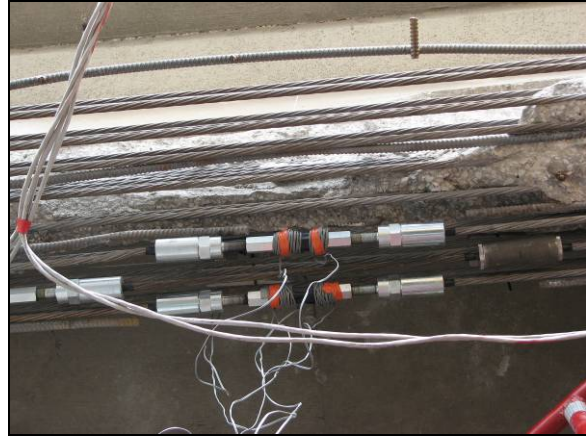
Fig. 11: Instrumented Mechanical Couplers
