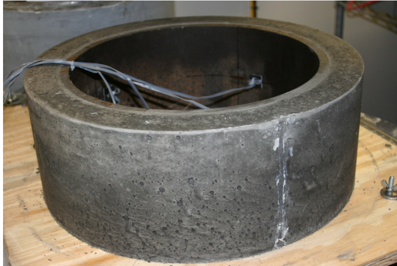
Figure 5 – Typical Shrinkage Ring
