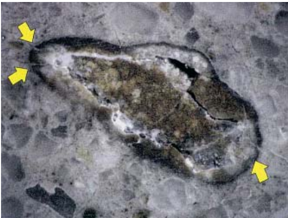
Fig. 10 Petrographic Analysis Showing ASR Gel
