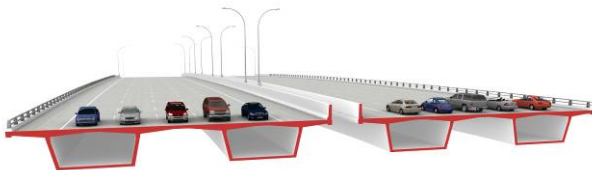
Figure 2 – I-35W Bridge Cross-Section
