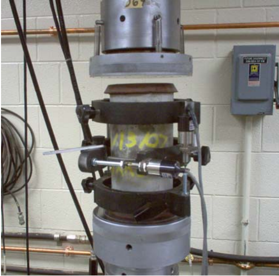
Figure 4: Apparatus and setup to measure elastic modulus of concrete cylinders
