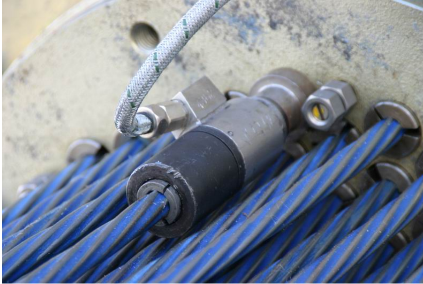
Fig. 19 Master strand load cell.
