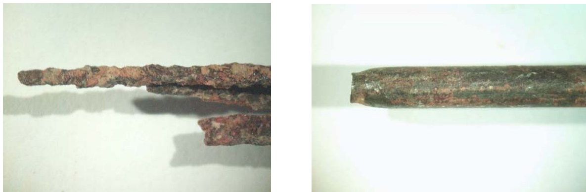
Figure 7 - Prestressing Wires Corrosion Failure (left) and Tension Failure (right)
