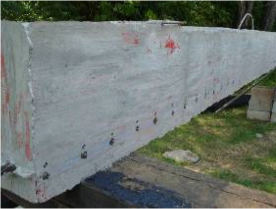
Fig. 8 DEMEC Target Locations
