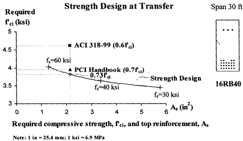
**Figure 1: Results of the strength design approach for the PCI standard 16RB40**<sup>11</sup>
