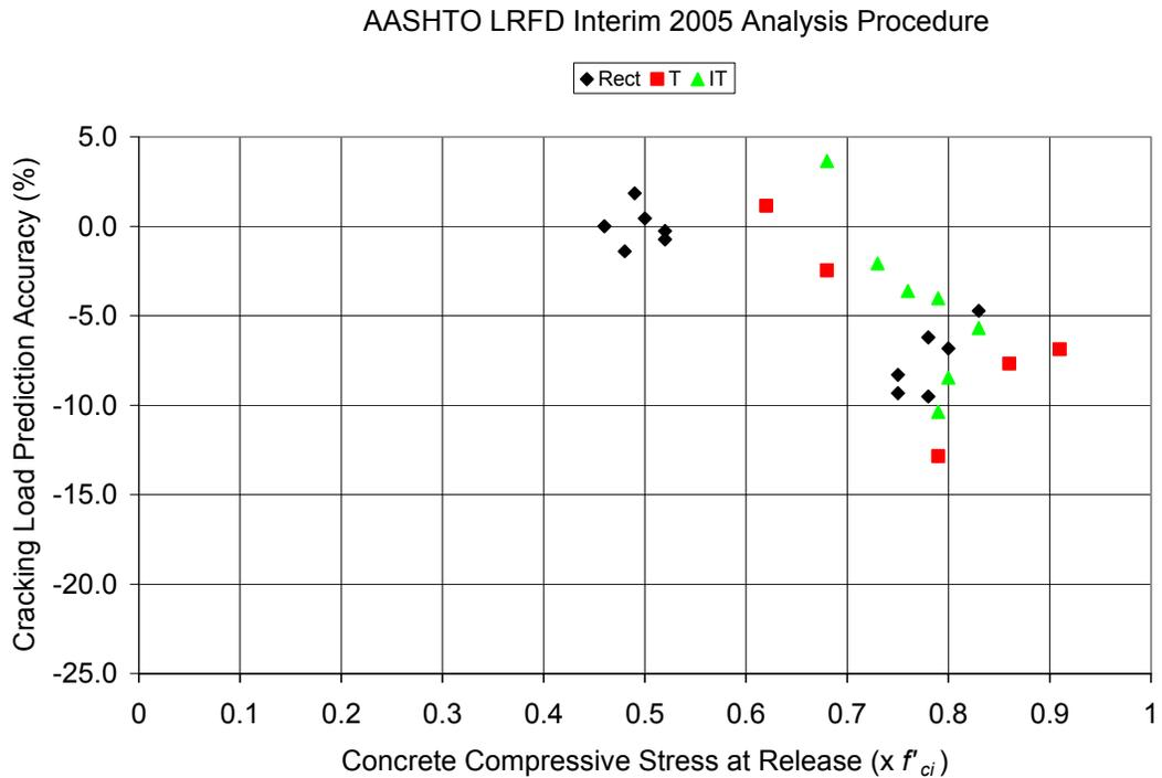
**Figure 11: Comparison of measured to predicted cracking loads using AASHTO procedure**
