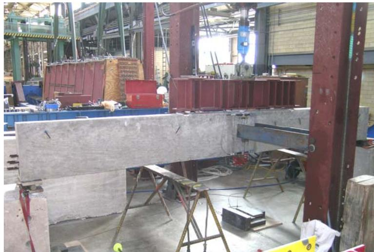
**Figure 7: Picture of static test setup for scaled girders**
