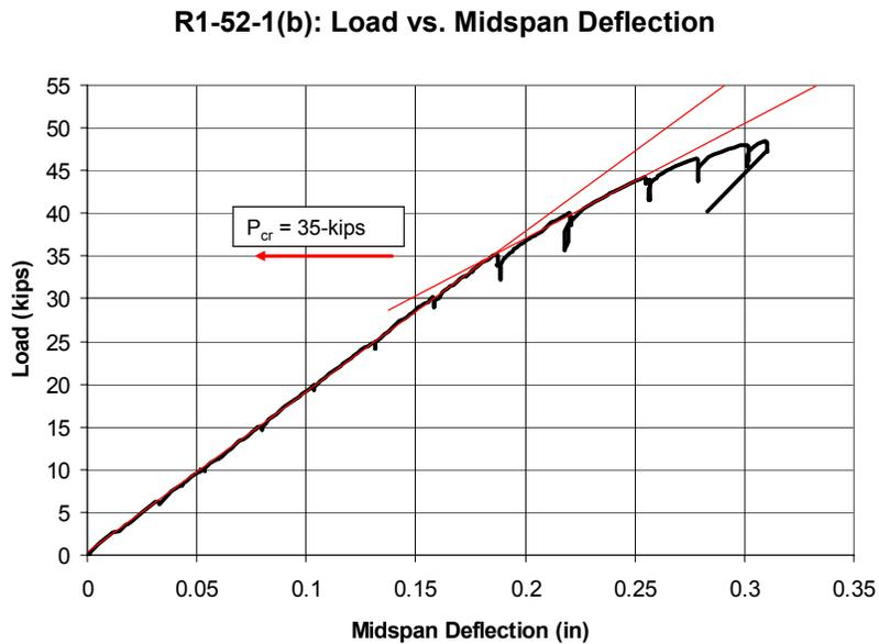
**Figure 8: Sample load versus midspan deflection plot**
