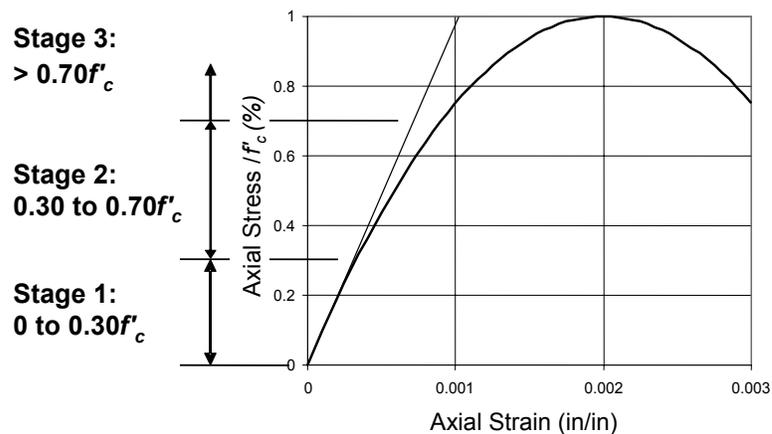
Figure 3: Illustration of findings of Hsu et al.<sup>17</sup> using concrete model of Hognestad<sup>18</sup>
