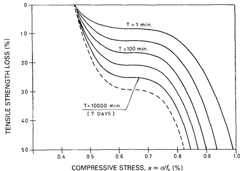
**Figure 4: Summary of tensile strength loss for typical concrete and curing conditions<sup>19</sup>**
