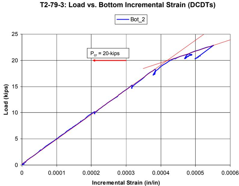
**Figure 9: Sample load versus bottom strain (1-inch from extreme fiber) plot**
