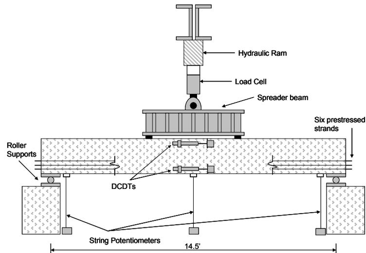
**Figure 6: Test setup for static load testing of scaled girders**
