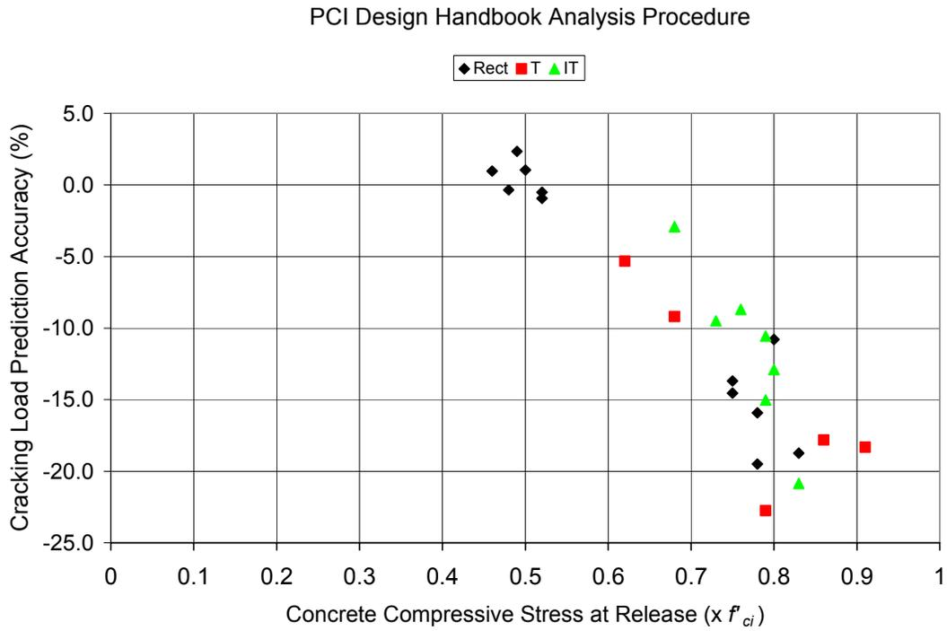
**Figure 10: Comparison of measured to predicted cracking loads using PCI procedure**
