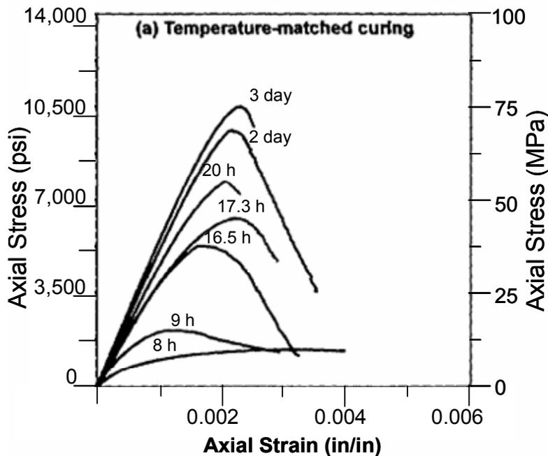
Figure 2: Stress-strain curves for a 10,000-psi concrete mix at various ages<sup>15</sup>
