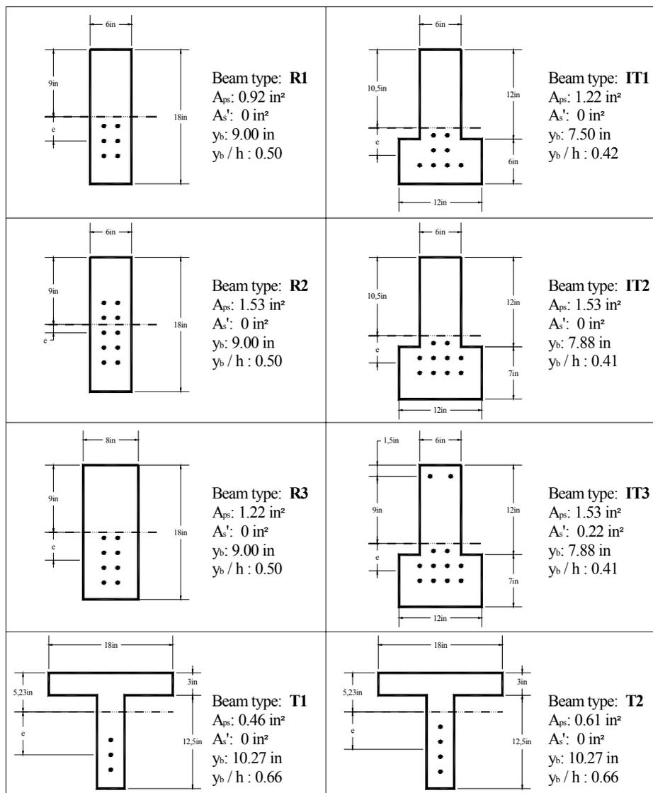
Figure 5: Different beam types fabricated in Project 4086<sup>12</sup>
