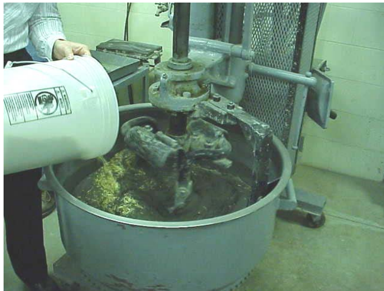
Figure 5. Mixing of UHPC
