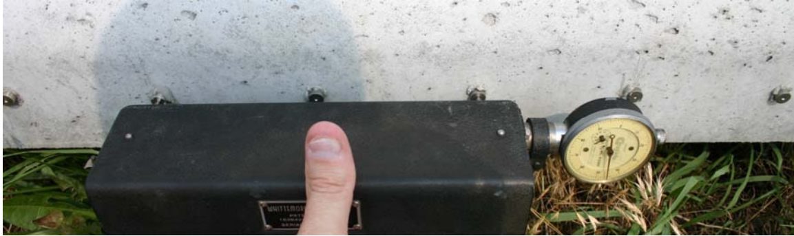
Fig. 4 Measuring concrete surface displacements with a Whittemore gage
