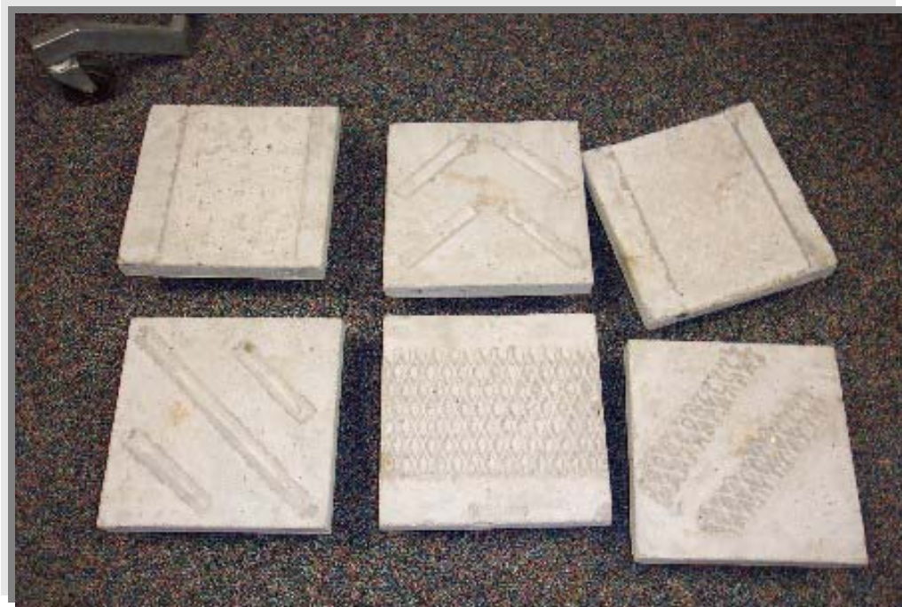
Figure 8. Roughened Surface Samples. Forming descriptions starting at the top, left going clockwise are: ball peen dented form, angle blockouts attached to form - variation 1, raised pattern plate metal form, angle blockouts attached to form - variation 2, metal lath form liner - variation 1, and metal lath form liner - variation 2.
