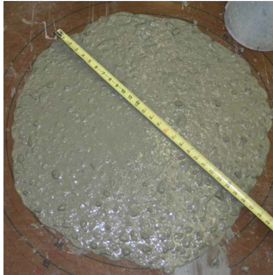
Fig. 2 Spread Test for SCC
