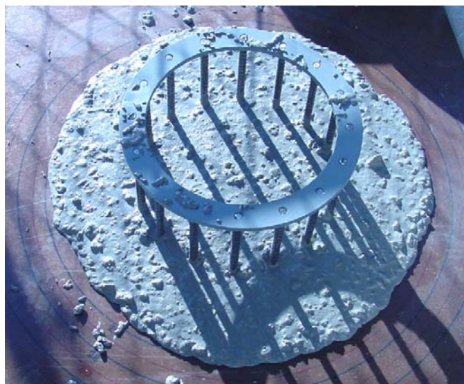
Fig. 3 J-Ring test for SCC
