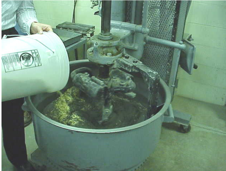
Figure 4. Addition of steel fibers
