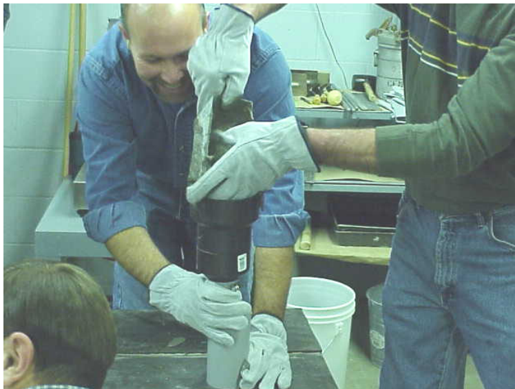
Figure 5. Casting of 3 inch x 6 inch test cylinders
