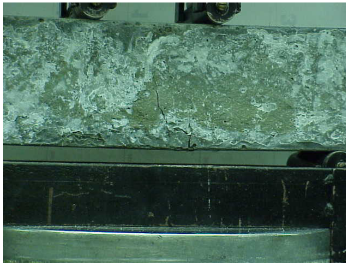
Figure 8. Failed 4 inch x 4 inch x 18 inch test beam
