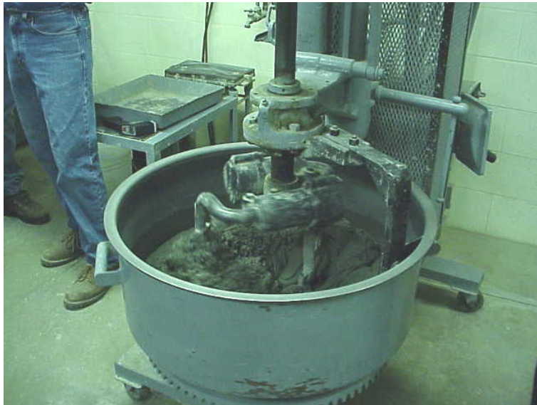
Figure 3. Mixing of UHPC
