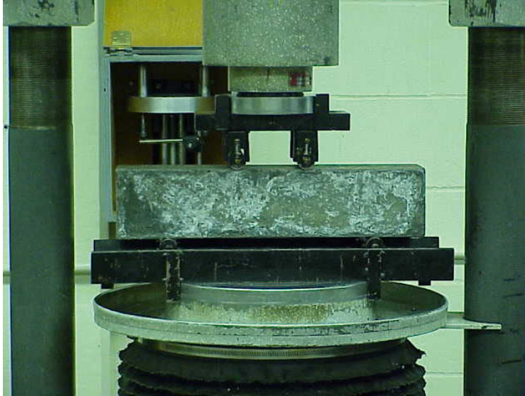
Figure 7. 4 inch x 4 inch x 18 inch flexure beam
