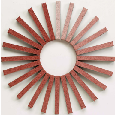
Synthetic Red Iron Oxide Pigment Additions from ¼% to 6% in white cement. Note how the last several samples look virtually the same. This is at or near the saturation point for this pigment.
