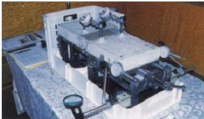
Fig. 3 Test Rig to Simulate Cracking (University of Bologna)
