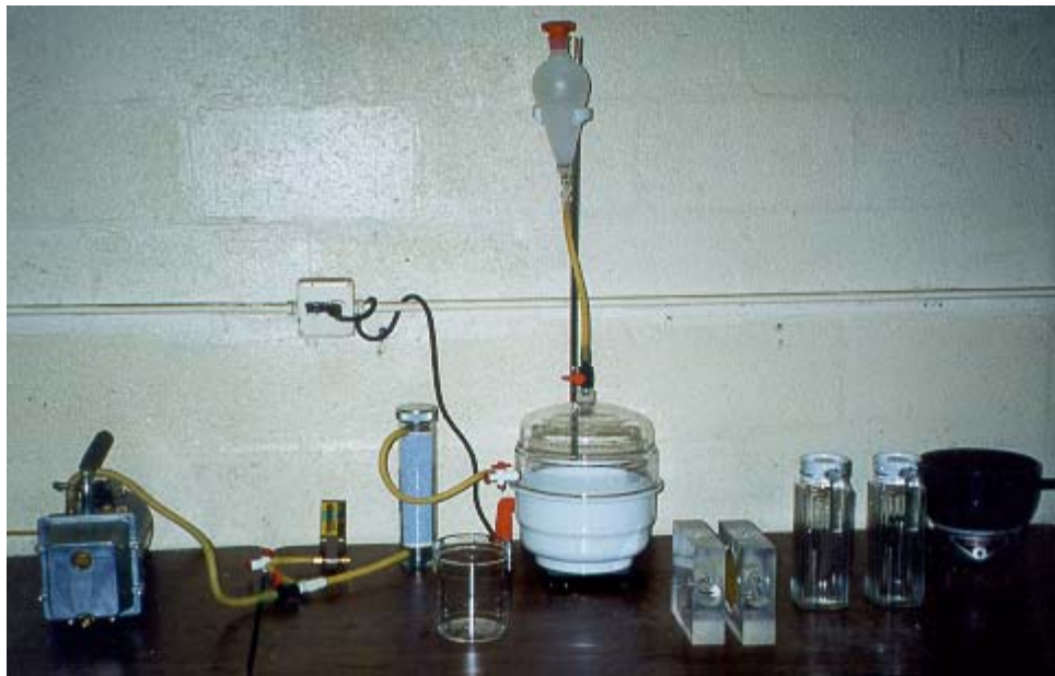
Fig. 2 Pump system for the permeability cell
