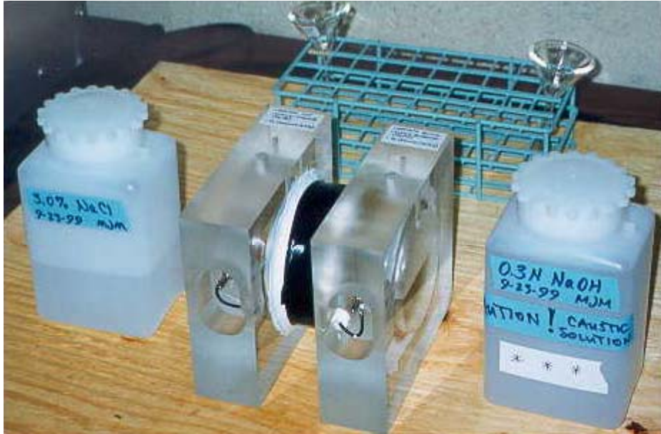
Fig. 3 Permeability cell ready for test
