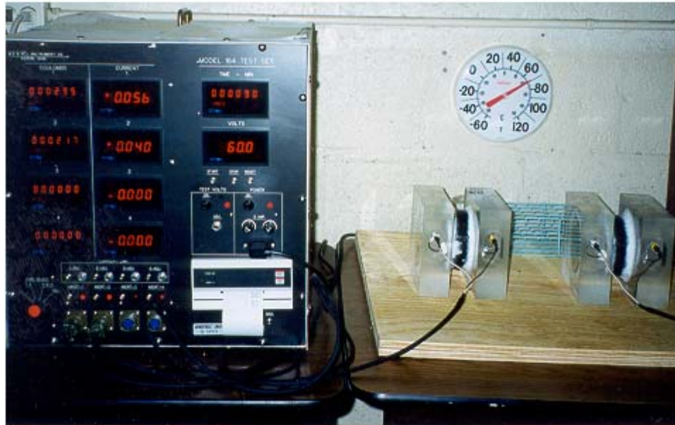
Fig. 4 Setup for permeability test
