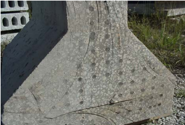
Fig. 3 Saw-cut cross section
