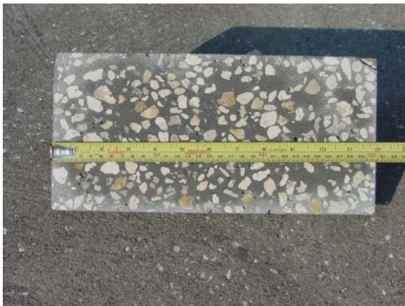
Fig. 5 Coarse aggregate measurement along the length of the core sample
