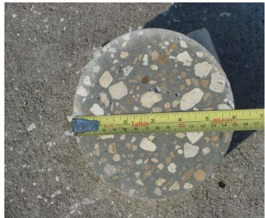
Fig. 6 Coarse aggregate measurement along the diameter of the core sample
