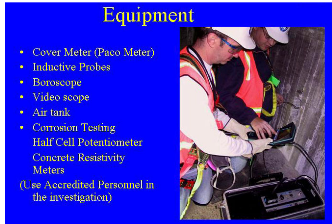
Fig. 11: Visual inspection equipment
