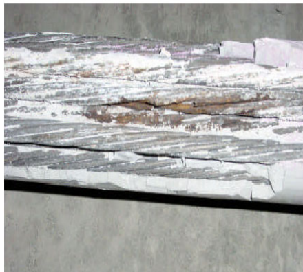
Fig. 5 Strand Corrosion from Cracked PE Duct
