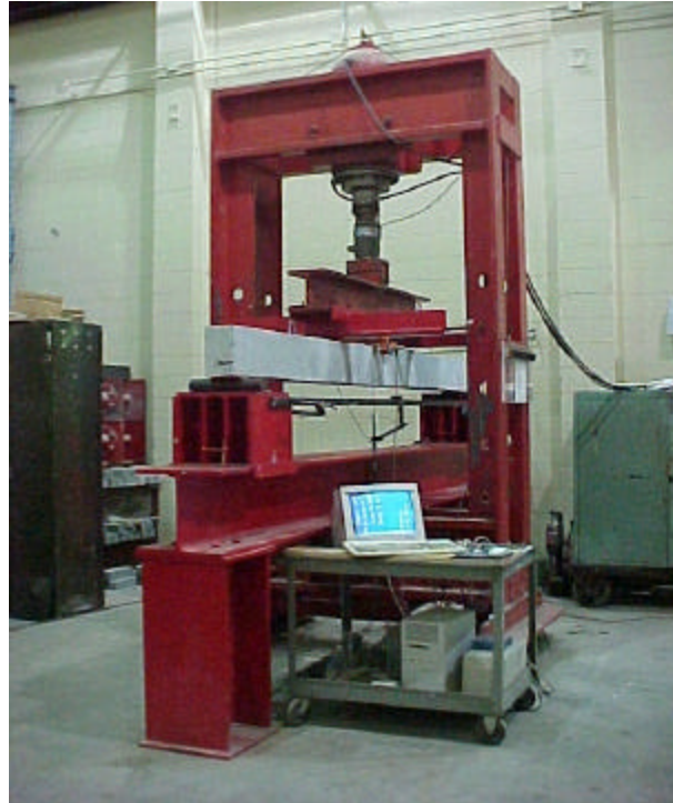
Fig. 2–Overview of Loading Frame for Testing of the Beam Specimens
