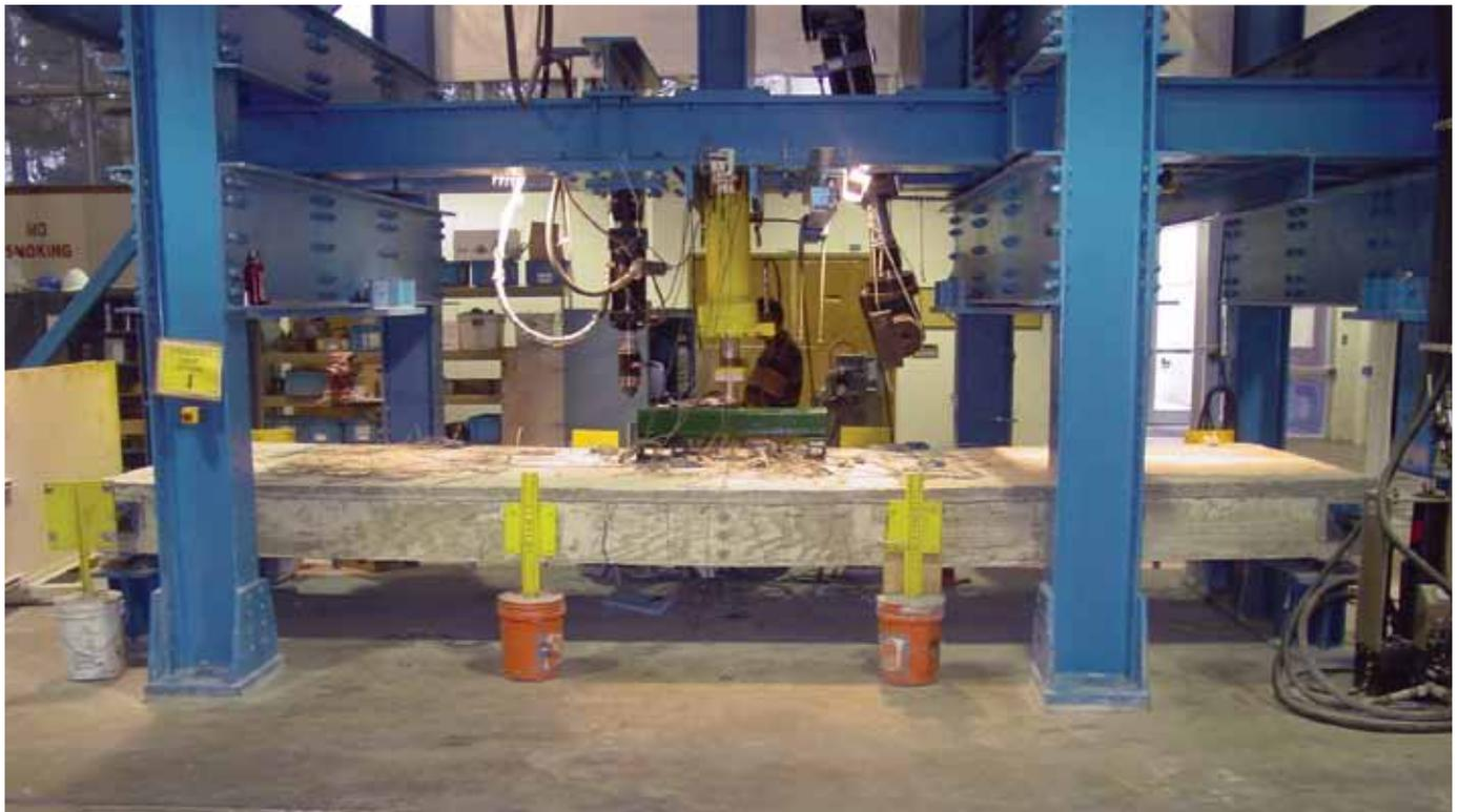
**Figure 4.** Load setup for the experimental model and crack development in the experimental bridge model under a load of 80 kip (360 kN).
