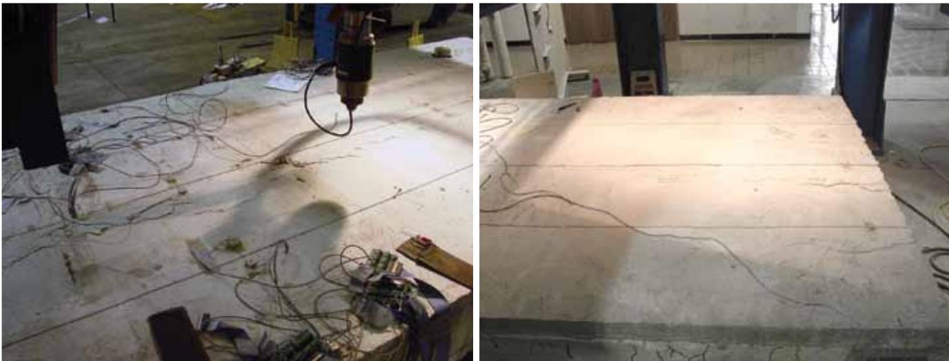
**Figure 5.** Midspan crack development and end-span crack development under a vertical load of 80 kip (360 kN) with no TPT force. Note: TPT = transverse post-tensioning.
