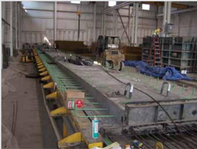
Minnesota inverted tee beam in precasting plant
