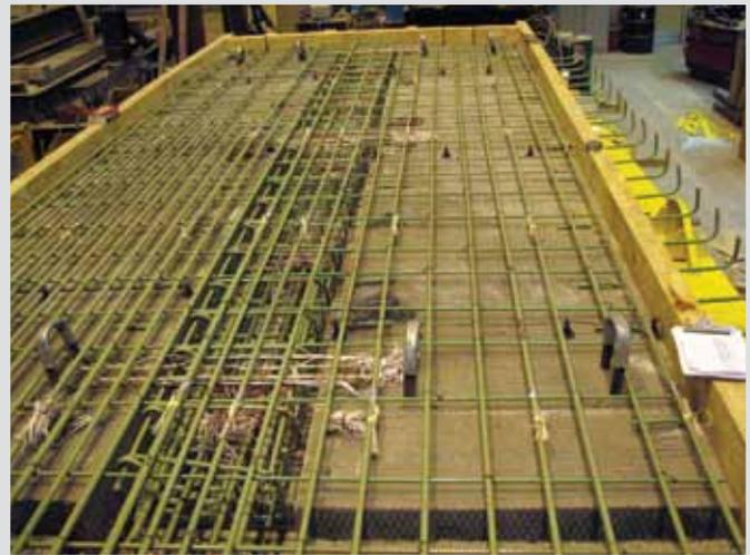
Deck and connection reinforcement for University of Minnesota specimens
