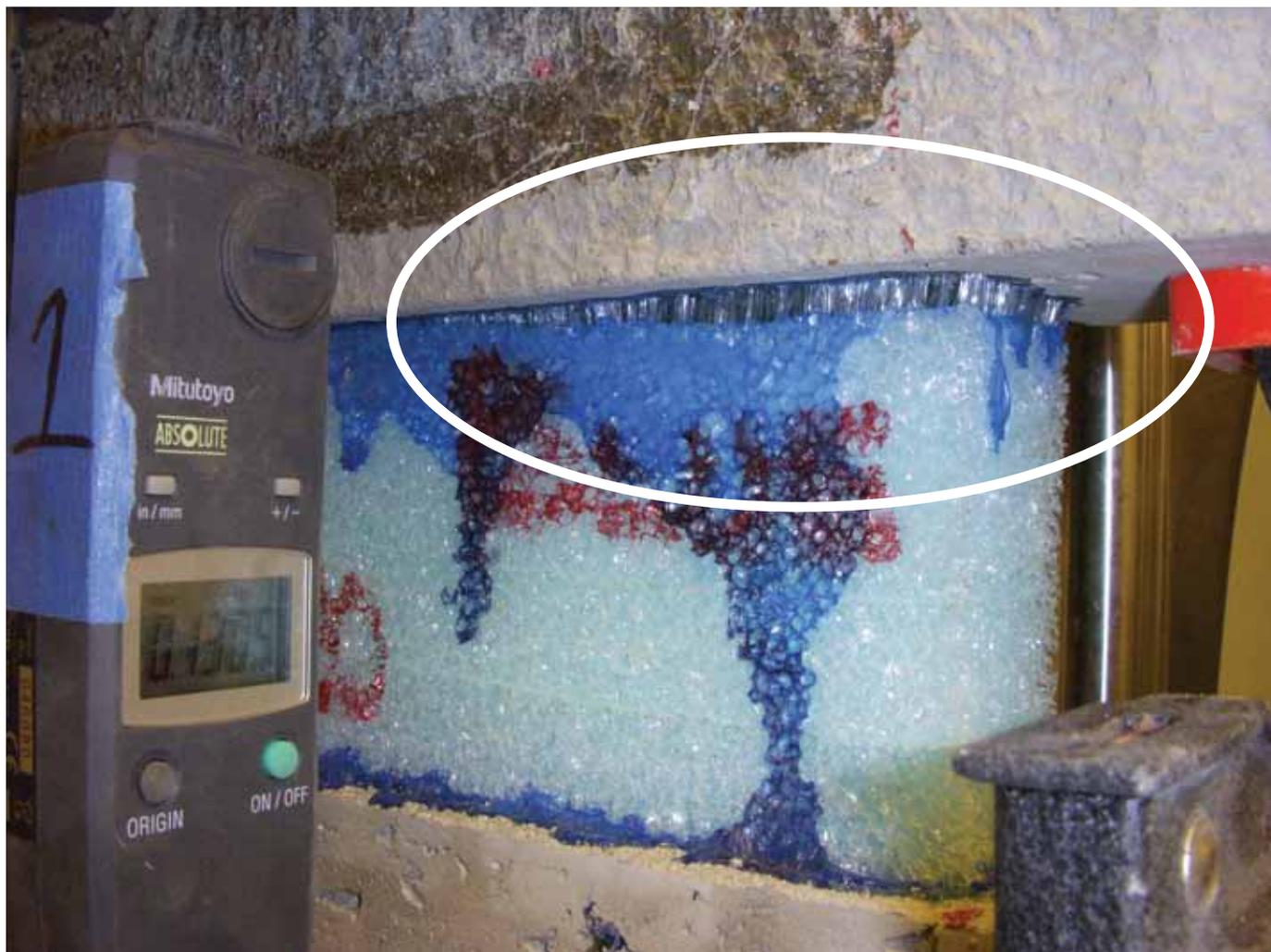
**Figure 7.** Failed specimen during tension test.
