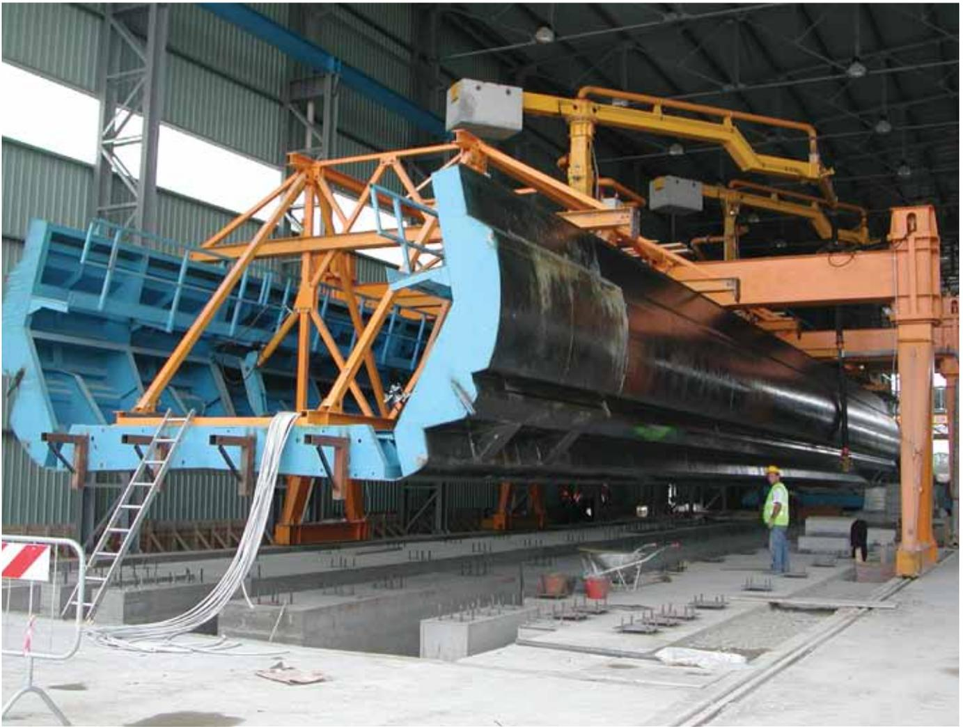
**Figure 3.** Movable interior form with concrete distribution arms.
