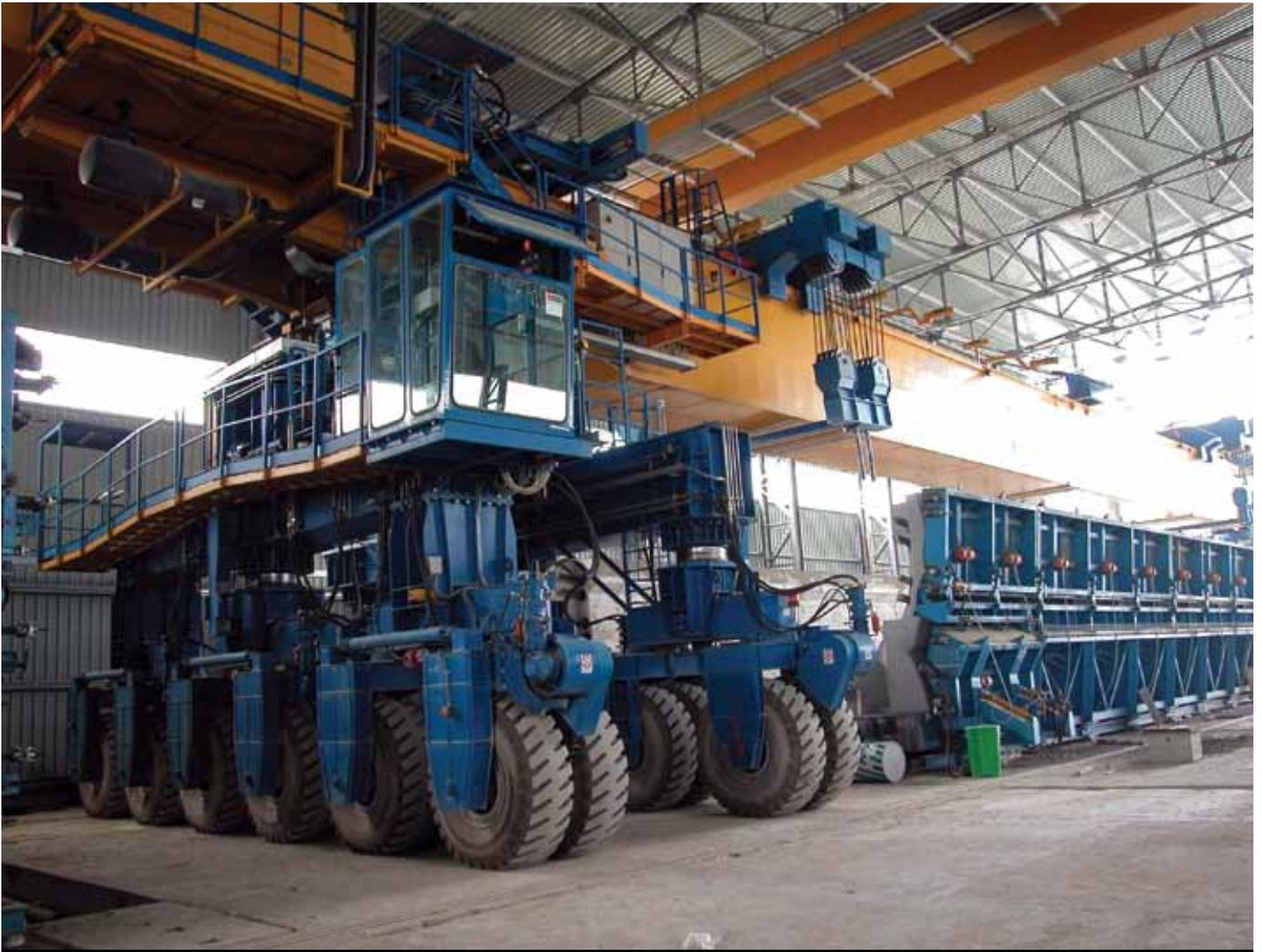
**Figure 5.** Span being lifted from the form.
