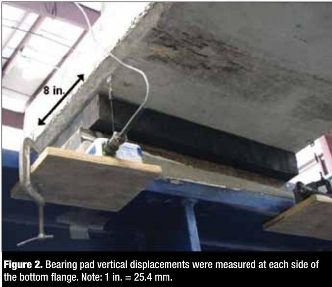
**Figure 2.** Bearing pad vertical displacements were measured at each side of the bottom flange. Note: 1 in. = 25.4 mm.
