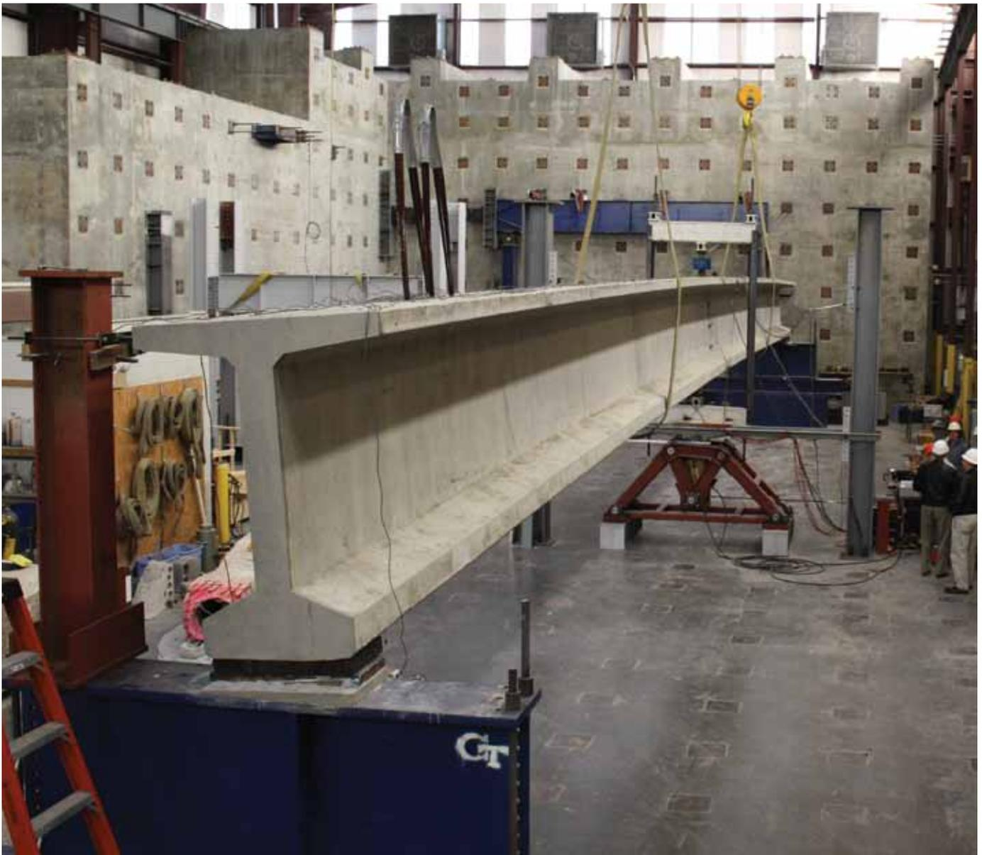
**Figure 1.** PCI BT-54 rollover stability experimental setup.
