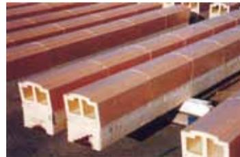
Glazes are covered by ASTM C126 and are tested in accordance with ASTM C67. Because glazed units have very low permeance to water vapor, it is recommended that a vapor barrier be installed on the warm side of the wall.
