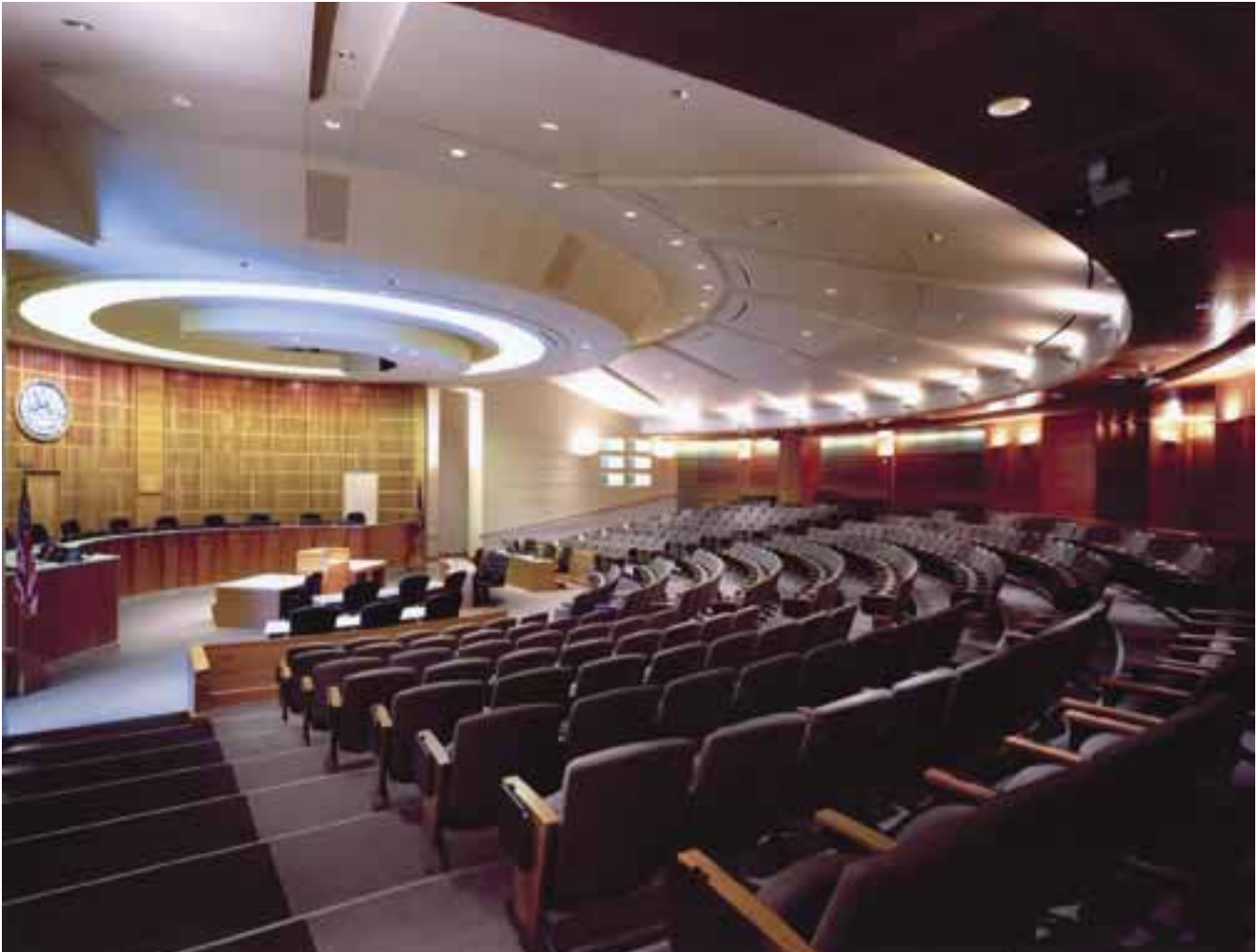
Fig. 5. The expansive open space in the City Council Chambers has 70 ft (21.3 m) spans, which are made possible by precast concrete double tees. [Photography courtesy of Michael Peck Studio]
