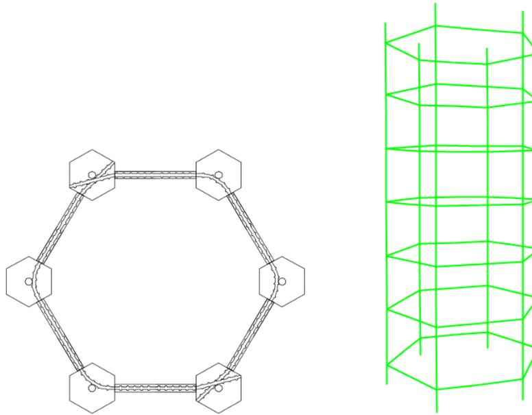
Figure 3: Radial tendon layout (left); radial and vertical tendon locations along test unit height (right)
