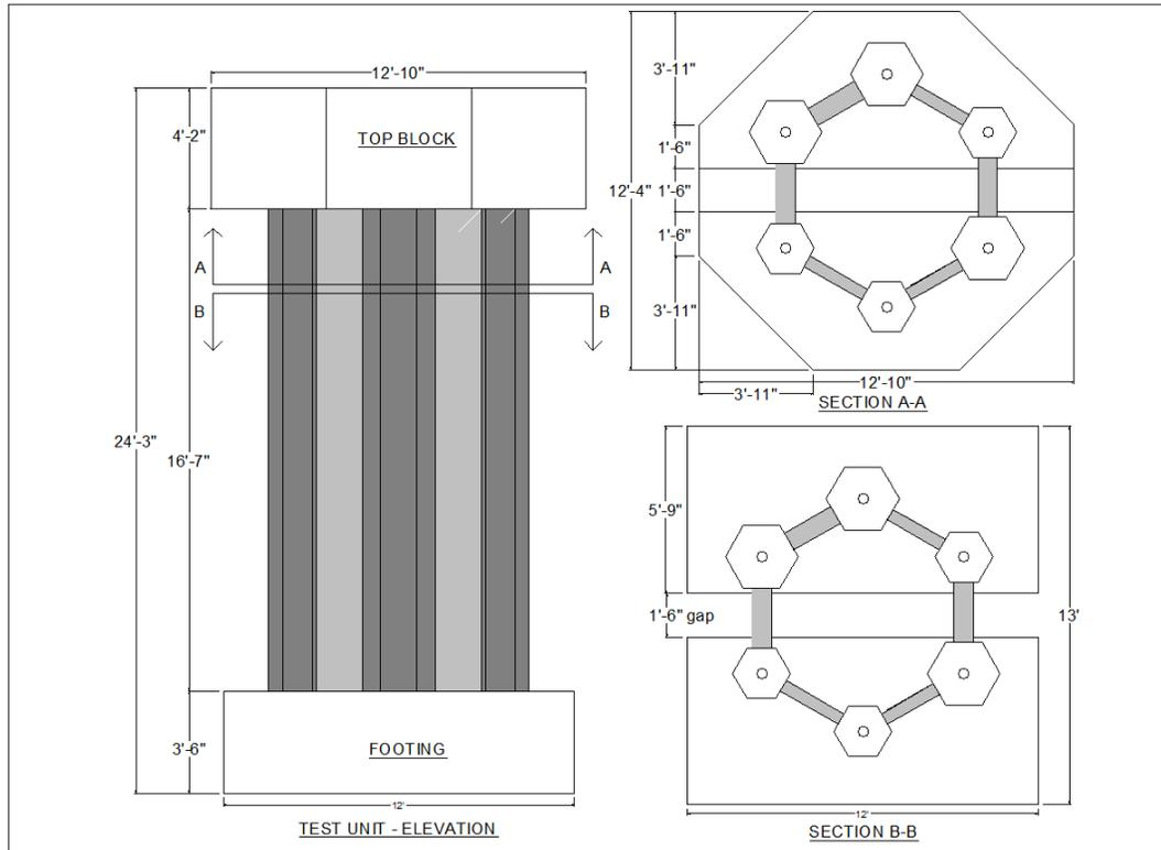
Figure 2: Test unit dimensions
