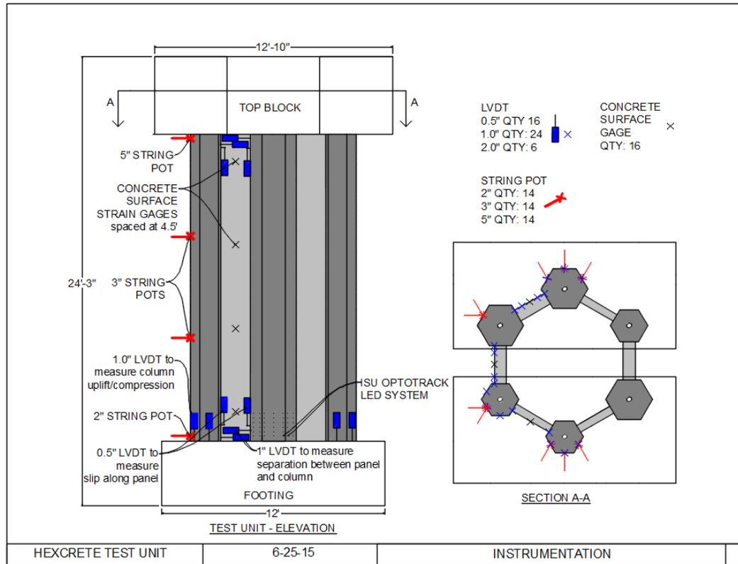
Figure 4: Instrumentation of test unit
