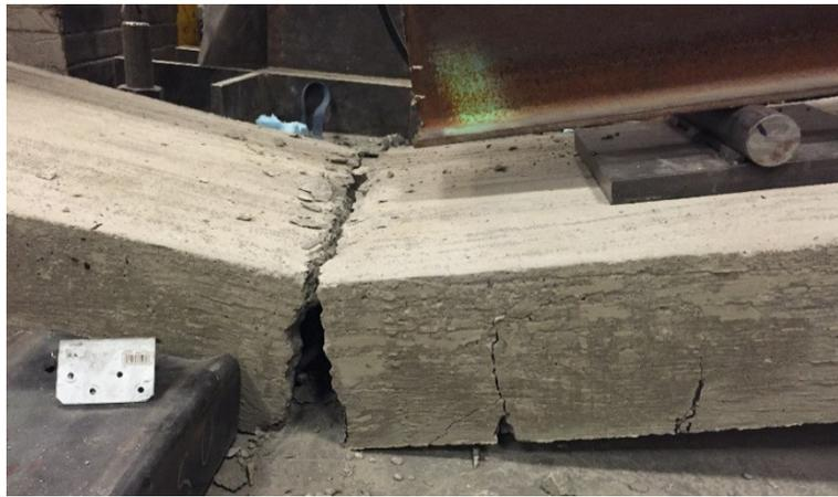
*Figure 7 – SW14 Ruptured Wire Failure*
