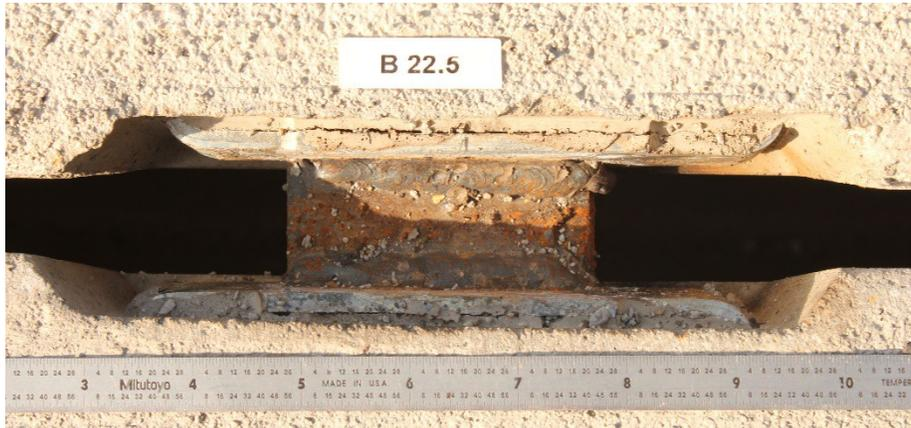
Figure 12: Typical Connection after Welding
