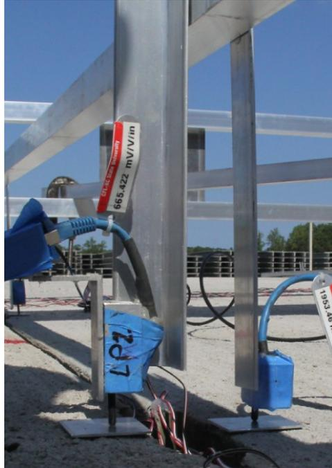
Figure 21: Typical Deflection Measurement at Typical Joint
