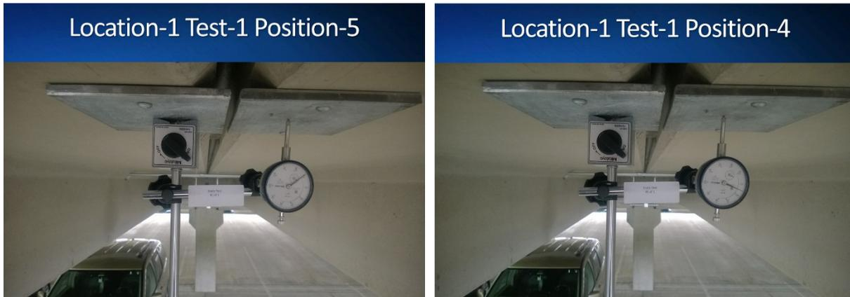
Figure 6: Test in Henrico, VA. In these photos, wheel to left of joint causes relative displacement 0.011 in. Wheel to right of joint causes relative displacement of -0.005 in.
