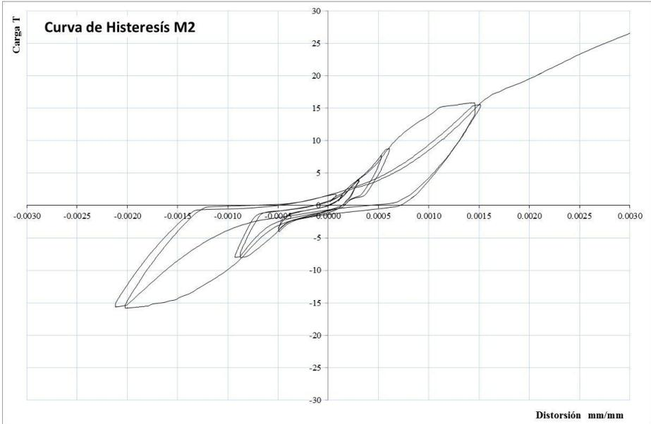
Wall behavior during the first cycles, maintaining the rigidity of the wall, as load increased, remarkable deformation is presented with this specimen achieving greater energy dissipation, reflected in the higher cracking presented.
