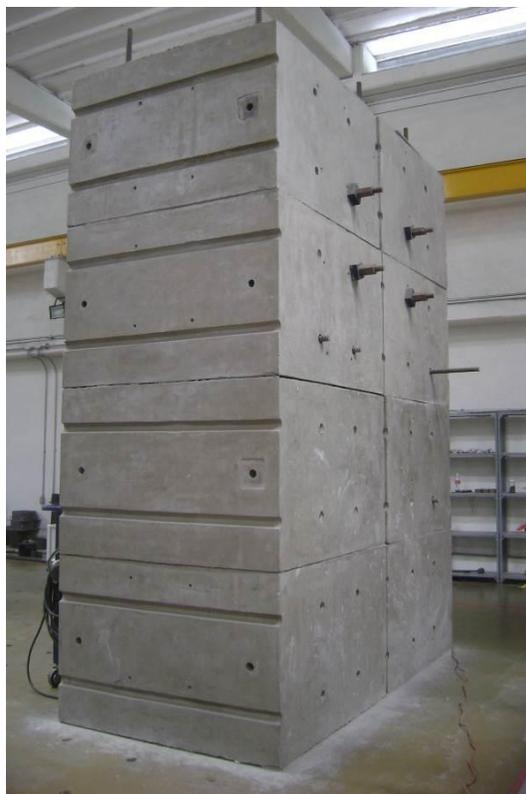
**Figure4 Wall reaction**
