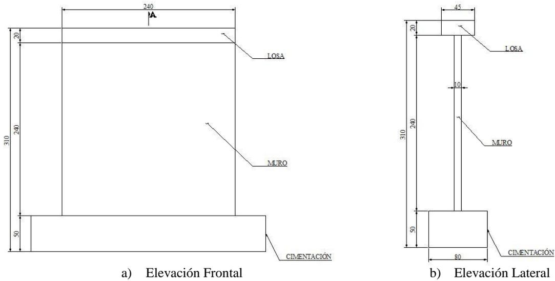
**Figure 7 Wall Geometry**
