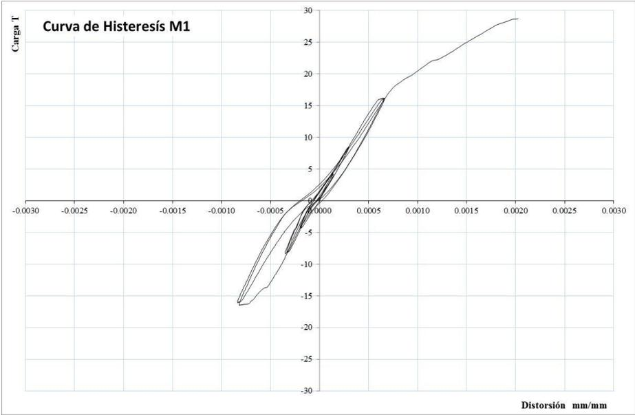
You can see that the behavior of the wall was rigid, because it retains the shape of the curves practically all rehearse, only up to a distortion of 0.0006, the stiffness changes, this is where there was greater wall cracking.
