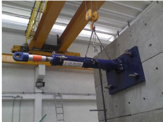
**Figure 3 hydraulic actuator ( 50 t)**
