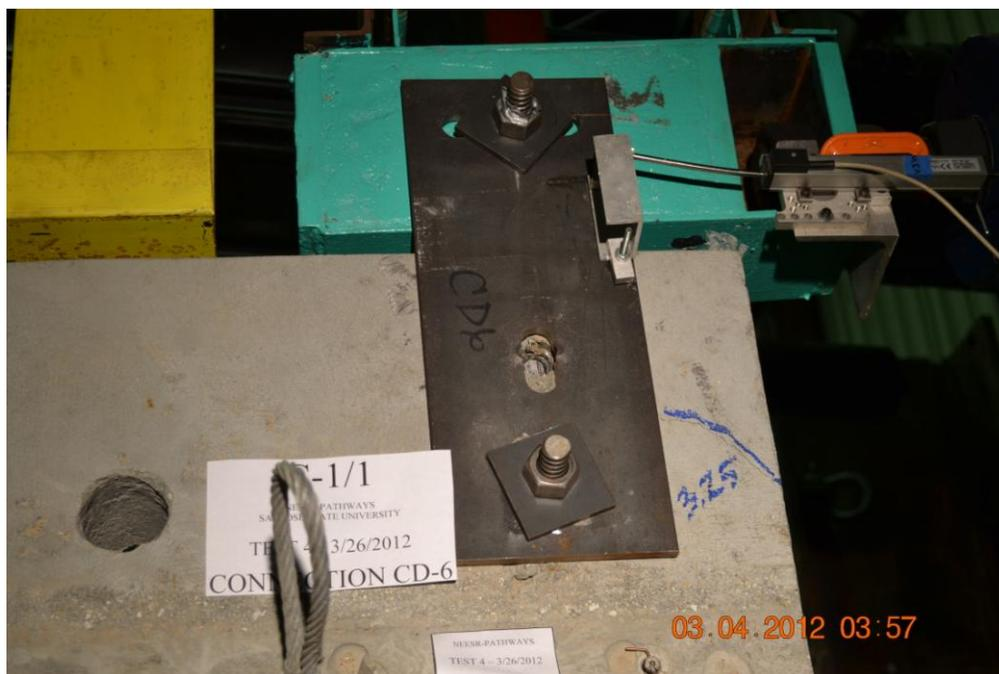
**Figure 1. Fracture of Coil Rod Supporting Plate for Slotted Connection (McMullin, 2013).**
