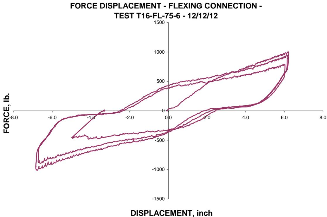
**Figure 6. Typical Force-Displacement Graph of  $\frac{3}{4}$ -inch Coil Rod Specimen with Length of 12 inches.**
