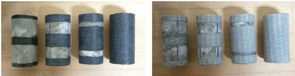
**Figure 1. Cylindrical Concrete Specimens Confined with CFRP (left) and GFRP (right).**
