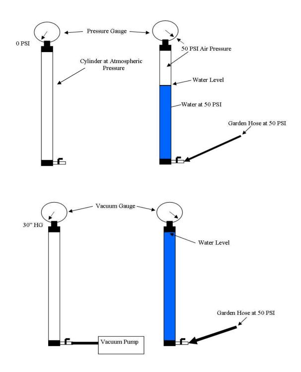
Fig 2 Proof is in this test- 10 foot clear PVC Tube is used to demonstrate the need to evacuate air to fill a void.
