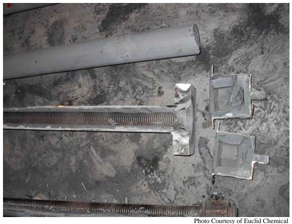
Fig 11. Cutaway of Sunshine Skyway test sample, loop tendon repair
