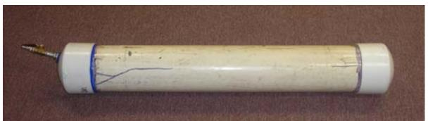
Fig 7 21.7 Liter Calibration Cylinder for Void Measuring Equipment (VME)
