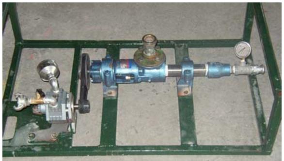
Fig 5 'Baby' Moyno- progressive cavity pump for vacuum grouting repairs
