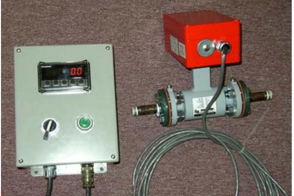
Fig 9. Grout Flow Meter- measures in liters or other standard units
