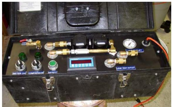
Fig 8. Forensic Void Measuring Equipment- contains system for pressurizing and detecting leaks
