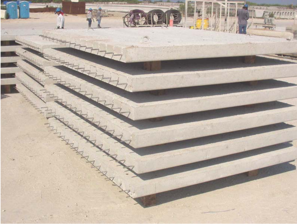
Fig. 7 Completed Panels in Storage – Note 3” Strand extension
