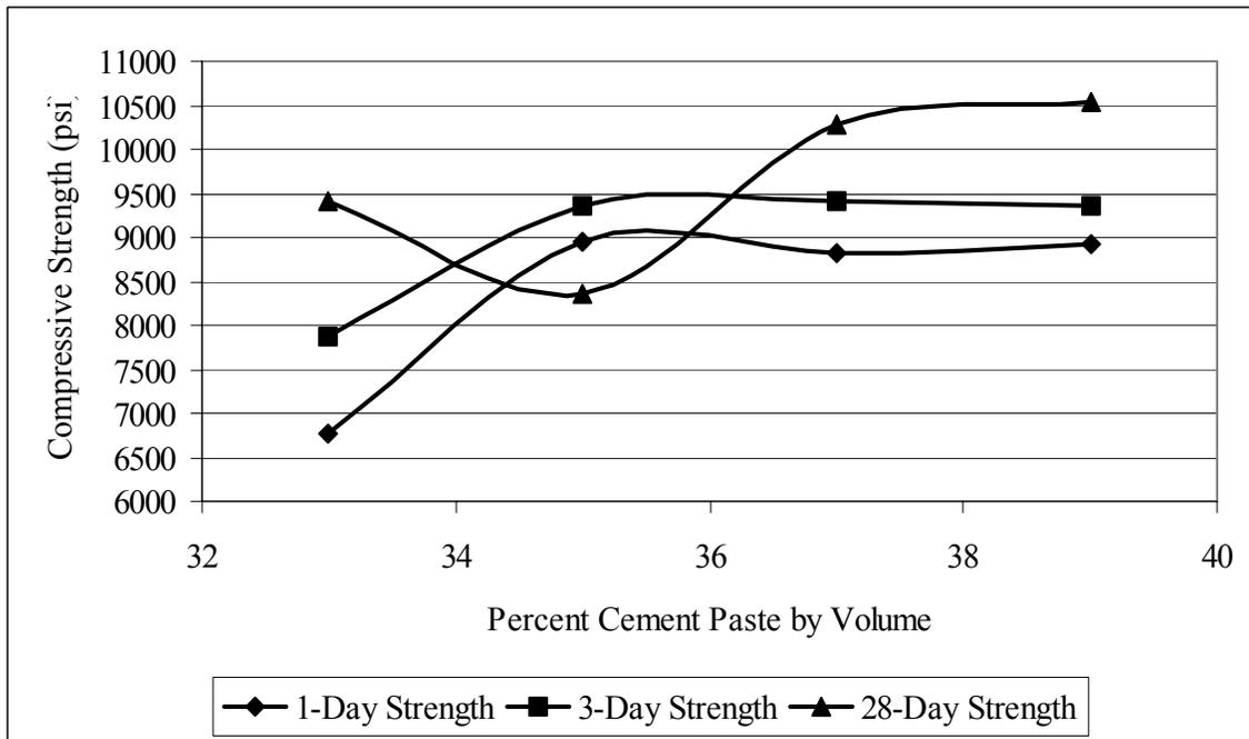
Figure 6. Results of Varying Percent Cement Paste
